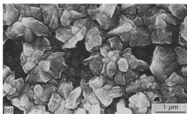
Fig. 11. SEM micrographs of the layer deposited from BE + CA. Time of second pulse: (a) 5, (b) 10 and (c) 20 s.
